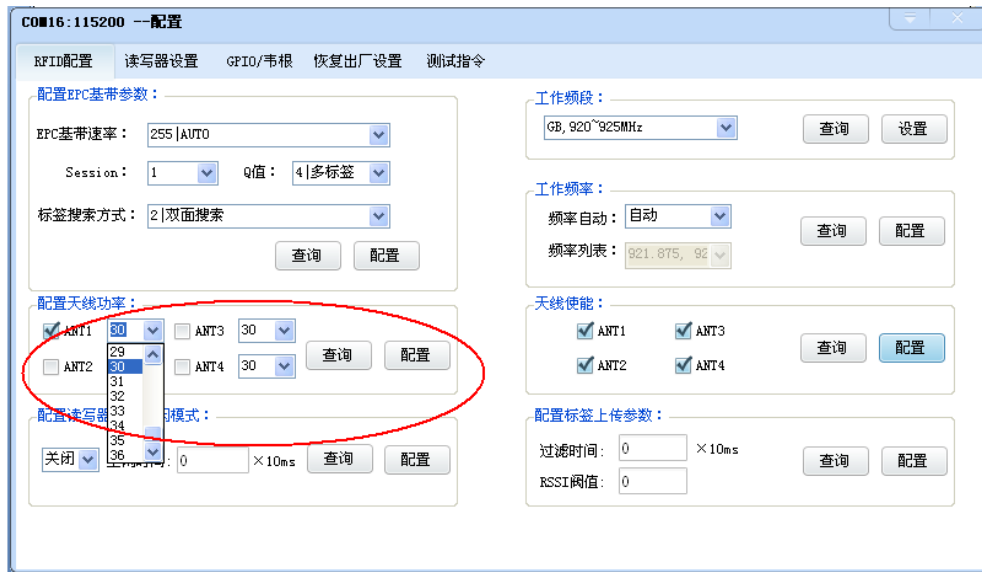
Image 4-22 Antenna port power setting
